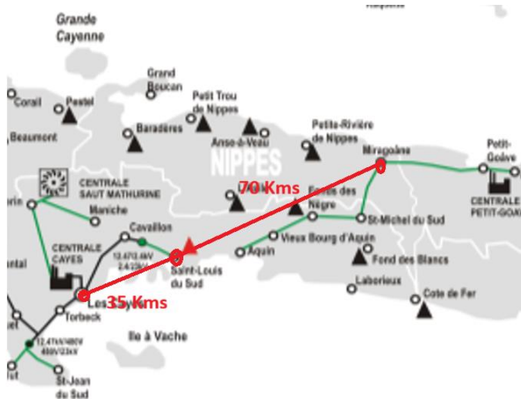
Figure 12 Regional Network 2 (RN2) – Reinforcement Plan
