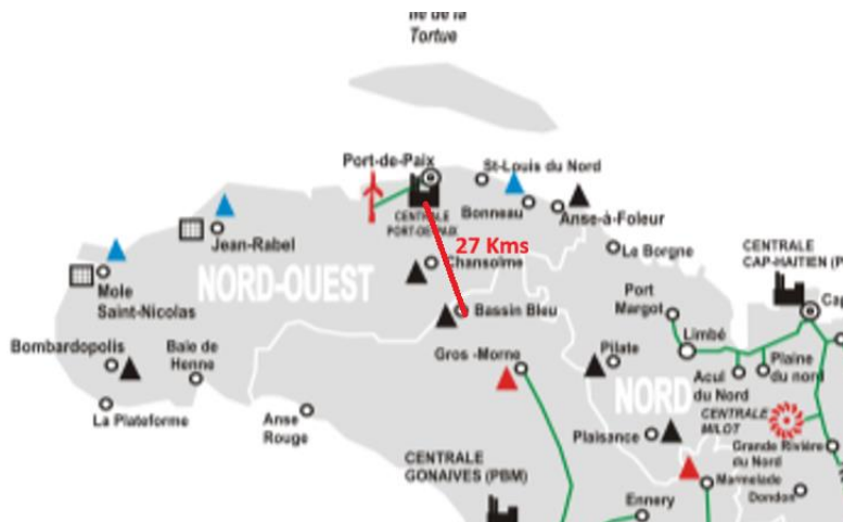
Figure 13 Regional Network 3 (RN3) - Reinforcement Plan
