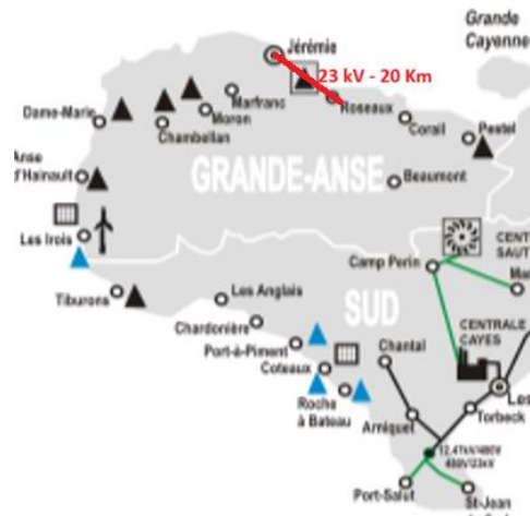
Figure 16 Regional Network 5 (RN5) - Reinforcement Plan
