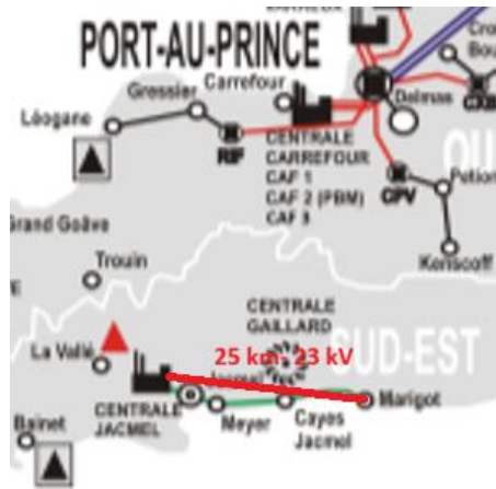
Figure 15 Regional Network 4 (RN4) - Reinforcement Plan
