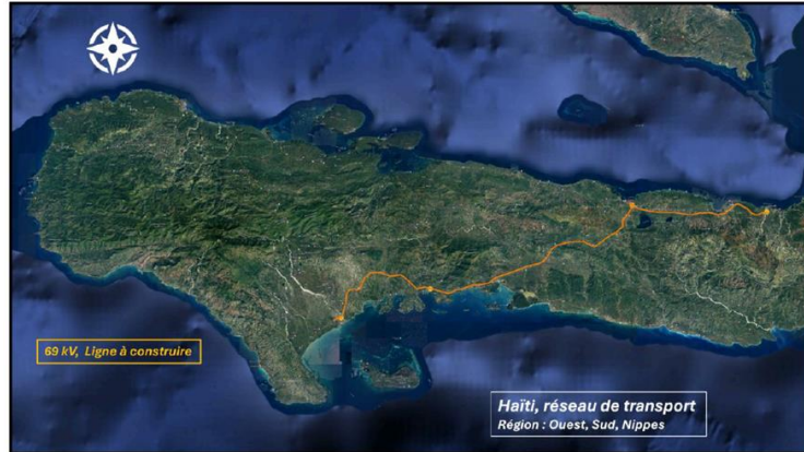
Figure 10 Illustrates the design of the transmission lines in region 2 MTPTC
